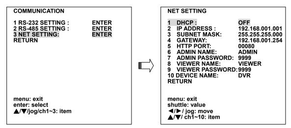
NOTE: If provided with a DHCP server, the 16CH DVR can get an IP automatically by setting the DHCP item to ON.
